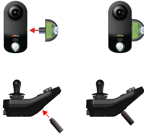
Figure 4: Inserting the LiNX Access Key (Above Top: low profile remote module. Above: traditional location)
